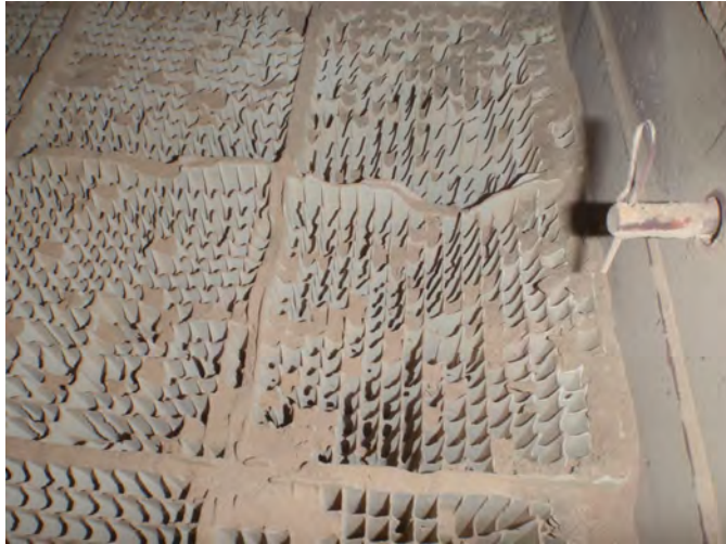
Moderate Erosion in L1 after 18,500 hrs
