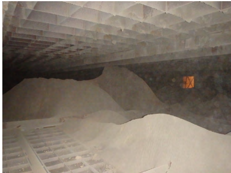
Larger Ash Piles From AIG to Far Side Through Center of Reactor
