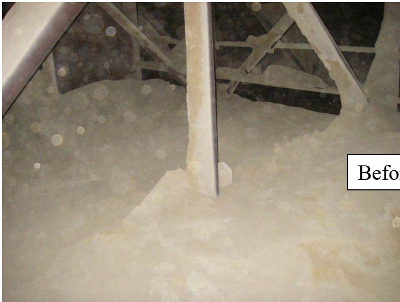
Moderate Erosion in L1 after 18,500 hrs
